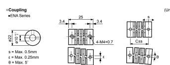
\*When mounting the coupling to encoder shaft, if there is big eccentricity or declination between rotating encoder shaft and mate shaft, it may shorten life cycle of the encoder or the coupling ※Do not load overweight on the shaft
