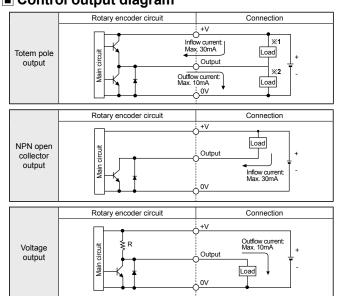
XThe output circuit of A. B. Z phase are the same ed for NPN open collector type(X1) or voltage output type(X2).
